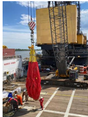
Armada Installer: Crane load test, working in the field, hammering works
